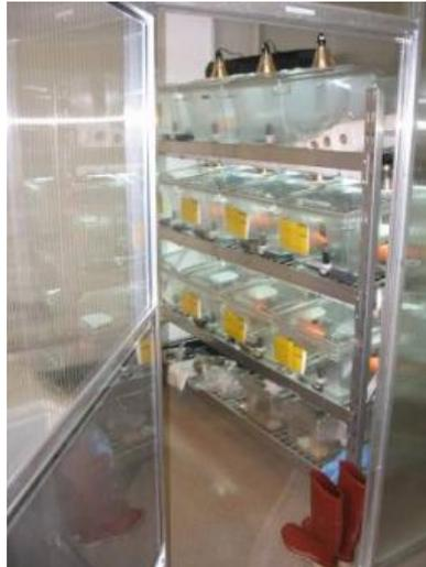
Figure 9. Lighting accommodated into the racks.
